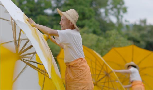
Although the modern umbrella industry has also entered the large-scale factory production, it still needs a significant amount of manual production. This is because of the specialty needed in making umbrellas. Manufacturing an umbrella involves assembling its vital components which include the shaft, a runner, stretchers, ribs, and a canopy.
